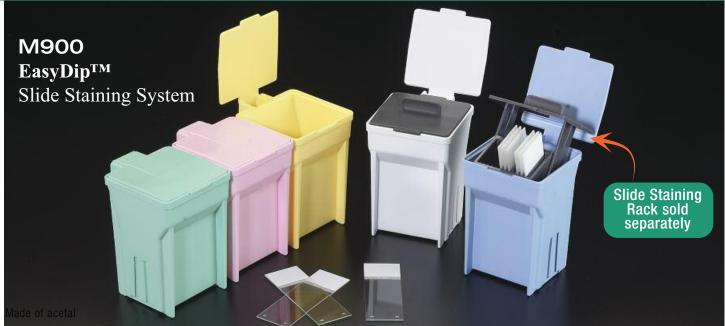
Finally a user-friendly approach for staining your microscope slides, the EasyDip™ Slide Staining System has two components: a square staining jar and a 12-position vertical slide rack. As an extra benefit, they are available in 5 different colors to help better identifying contents or applications.
